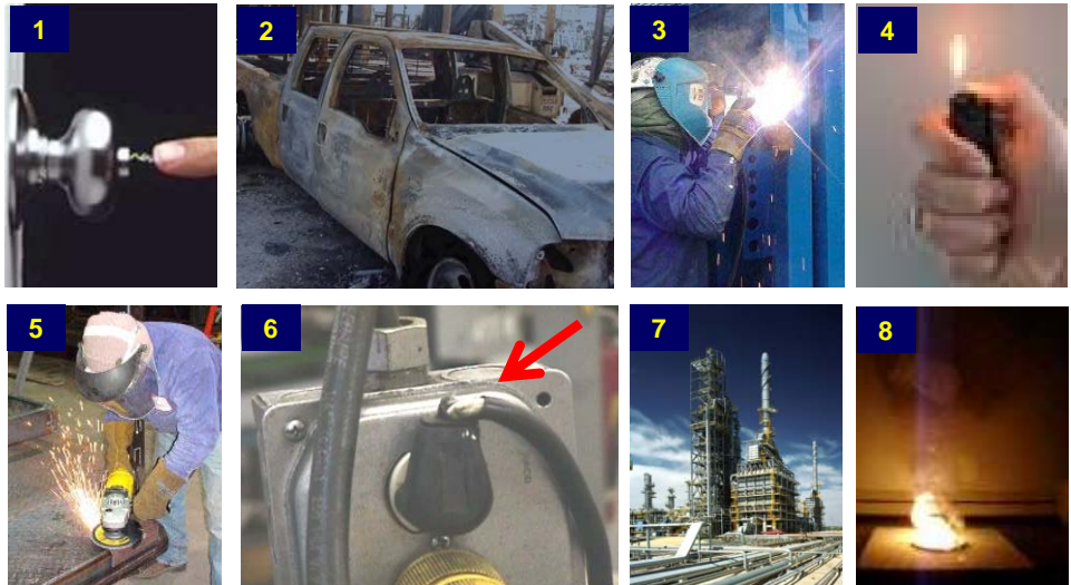
Some examples of ignition sources: (1) static electricity, (2) vehicle, (3) welding, (4) open flame, (5) grinding, (6) faulty electrical wiring, (7) a furnace, (8) pyrophoric or decomposing material
